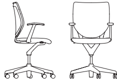
9313 Conference Chair, Upholstered With Arms, Pneumatic Height Adjustment W 24.5" D 21.25" H 37.25-41.5" SH 17.25-21.5" AH 26-30.25"
