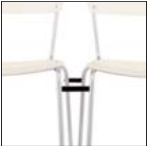
Optional ganging mechanism
